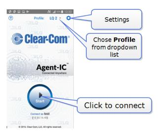
**Note:** When connecting Agent-IC to HelixNet via LQ, due to a heavier codec (WavPack), the data rate will increase. This may cause problems with the Agent-IC client in HelixNet Channels, particularly when using the slower 3G bandwidth connections.
