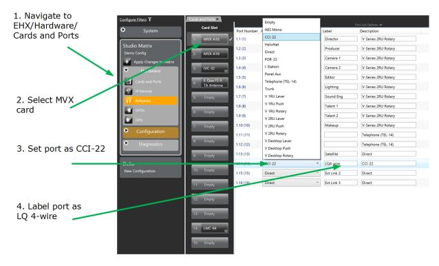
**Note:** The connection between the MVX or PiCo and the LQ device is a 4-wire connection, even though it is declared as a 2-wire connection.
