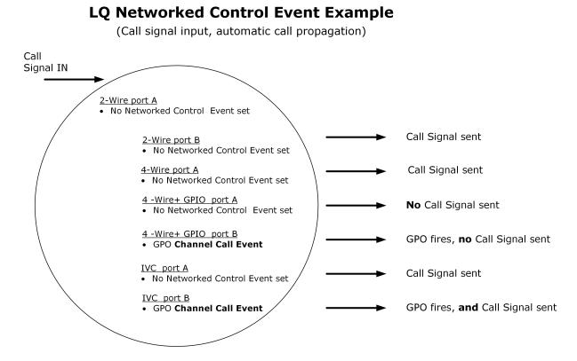
**Note:** Call signals are automatically propagated to all members of a Channel when using LQ so a GPI trigger is unecessary. However, a GPIO interface will not send a call signal trigger unless a GPO Call Channel event is set on that port.
