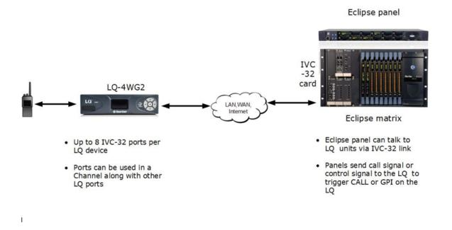
Each LQ-R unit supports up to 24 ports: 8 hardware ports, 8 SIP ports and 8 virtual ports. Agent- IC and IVC ports are considered 'virtual ' ports. Virtual ports can be used in any combination up to 8 in total.
