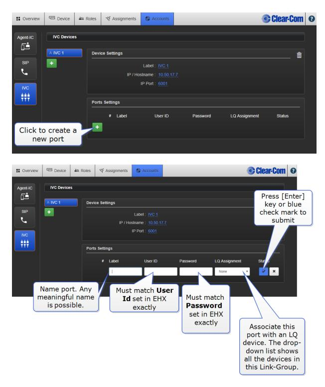
When the LQ is connected to the IVC-32 card, a green status LED shows. If the connection is not successful, a yellow warning displays. Click the yellow warning symbol for information.
