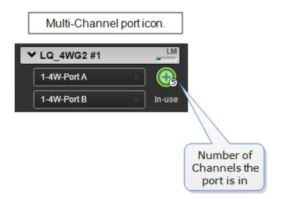
**Note:** If the port has already been put into a Channel, it will be unassigned from the Channel when you enable multi-Channel support.
