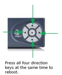
The system can also be rebooted using the front panel menu screens: **Menu > Administration > Reboot** and from the CCM: **Device > General > Maintenance > Reboot**.
