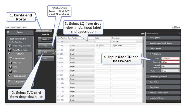
When you have set up the new ports, you must **Apply changes to Matrix**.
