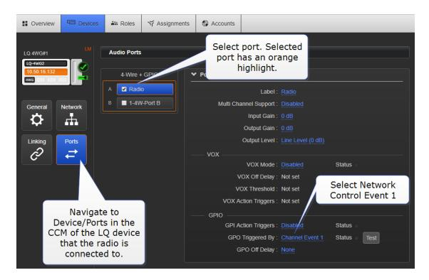
Once you have set up the ports, navigate to Assignments in the CCM and put ports into a Channel.
