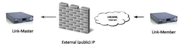
All devices within a Link-Group must have connectivity to the Link-Master on TCP port 80 (TCP port 433 if using the HTTPS protocol) and TCP/UDP port 655. When linking devices over the Internet, make sure that this connectivity is stable. Internet connection to an LQ device requires special configuration within your firewall (port-forwarding).
