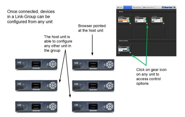
The Core Configuration Manager (CCM) for any LQ host can be accessed by entering the IP address as displayed on the front panel display of the LQ host into a web browser's address field. All devices in the Link-Group can be viewed and configured through any single host in the Link-Group.
