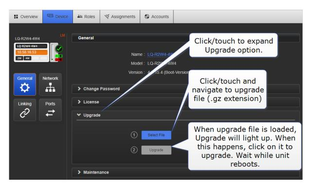
**Note:** If you downgrade an LQ unit from Version 2 to Version 1, you will see a red light flashing on the front panel after the first reboot. Power cycle the unit one more time to reset the status.
