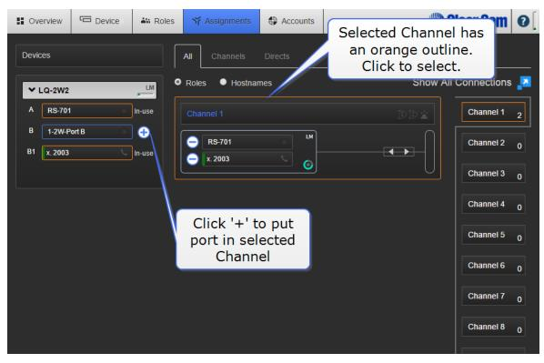
Audio sources are now connected in a Partyline (conference) setup. You can dial into Channel 1 from an external phone and dial out from Channel 1 using the CCM.
