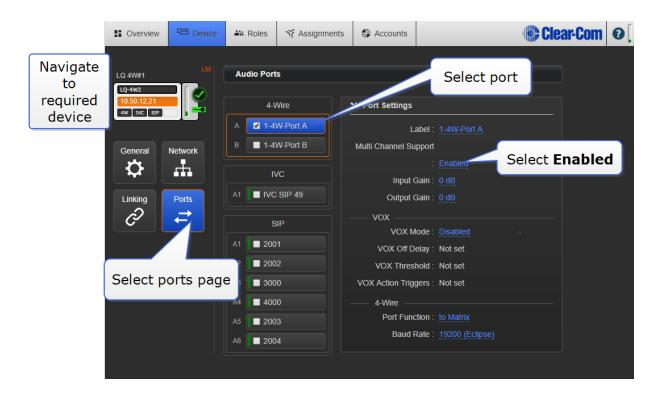
Once enabled, multi-Channel ports are available in the Assignments page, ready to be assigned to more than one Channel.
