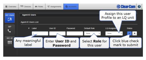
Your Agent-IC user profiles are now setup and the client device can chose a Profile and connect to the system.
