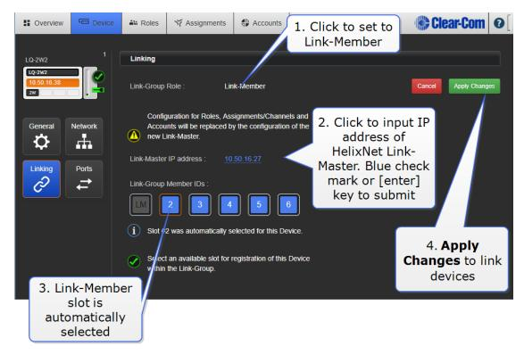
c. For each device to be added to the Link-Group, input the device IP into the browser's address field to access the CCM, designate the device as **Link-**
