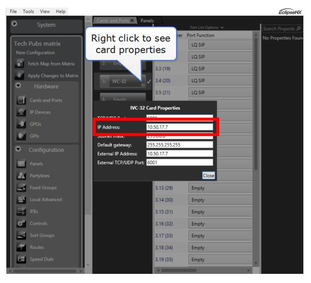
4. Generate IVC ports. Give the LQ unit the Username and Password already set up in the EHX software. Assign port to an LQ unit to connect.
