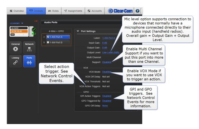
Note:A 4-wire+GPIO port will not transmit call signals in the form of data. The GPOOutput Trigger must be set to Channel Call Event, or a signal will not be sent.
