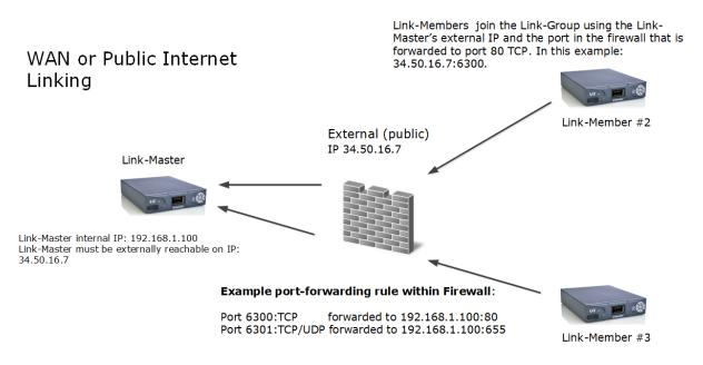
The Link-Master uses TCP port 80 for management and TCP/UDP port 655 for audio (it uses port 433 for management if you are using HTTPS rather than HTTP). You will need to create port-forwarding rules within your firewall to make these ports externally accessible to the Link-Master device.
