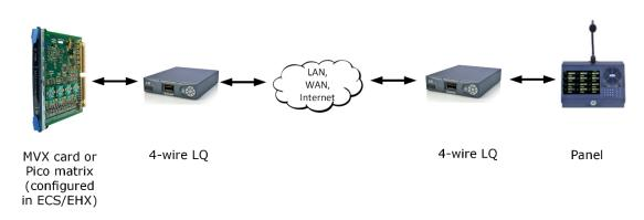
When setting up this connection, the MVX port to the LQ should be declared as a panel in the EHX software.
