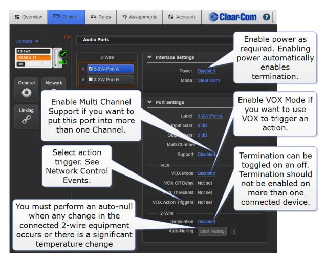
**Autonull**: You must perform auto-null when any change in the connected 2-wire equipment occurs or there is a significant temperature change.
