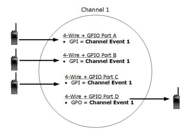
Example 4. Call Event trigger. Passing call signals using GPIO
