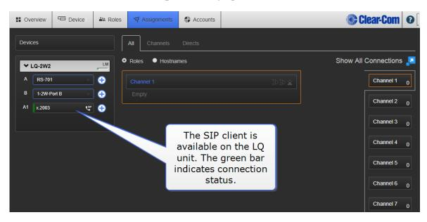
5. Go to the **Assignments** page of the CCM. Bring both the External port and the SIP port together in a **Channel**.
