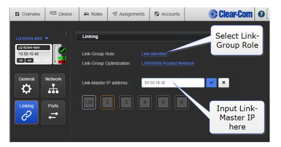
To take an LQ device out of a Link-Group, change it's role back to Link-Master here. This will disconnect the device from the group.
