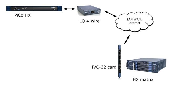
For this set up it is necessary to configure both EHX and the Core Configuration Manager (CCM).
