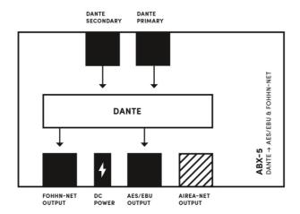
In this operating mode, the AIREA-NET output must not be connected to anything!
